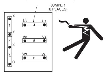
Figure 15. Voltage Change-Over Board 240V Configuration
